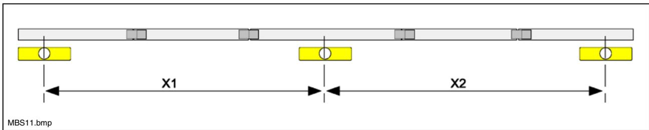
The distances between the sensors are ideally identical ( $X1 = X2$ ).
