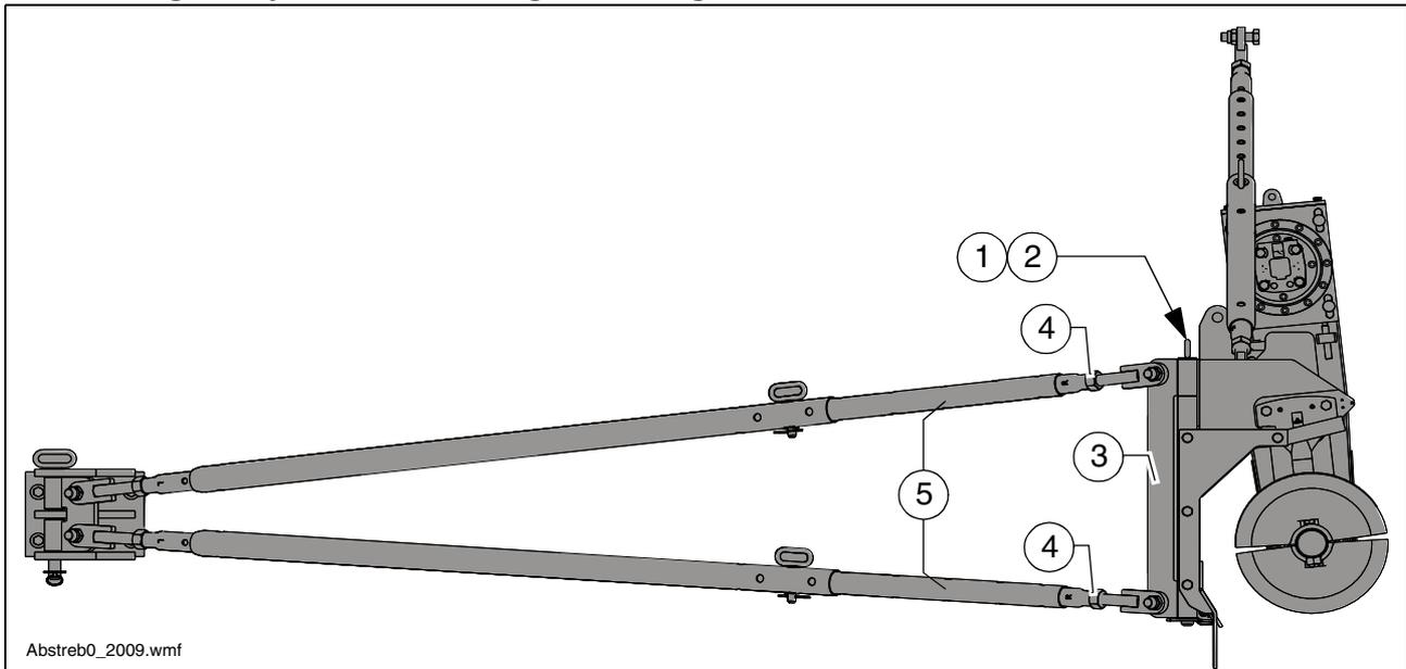
Auger height adjustment for large working widths can be carried out with a hinged brace:
