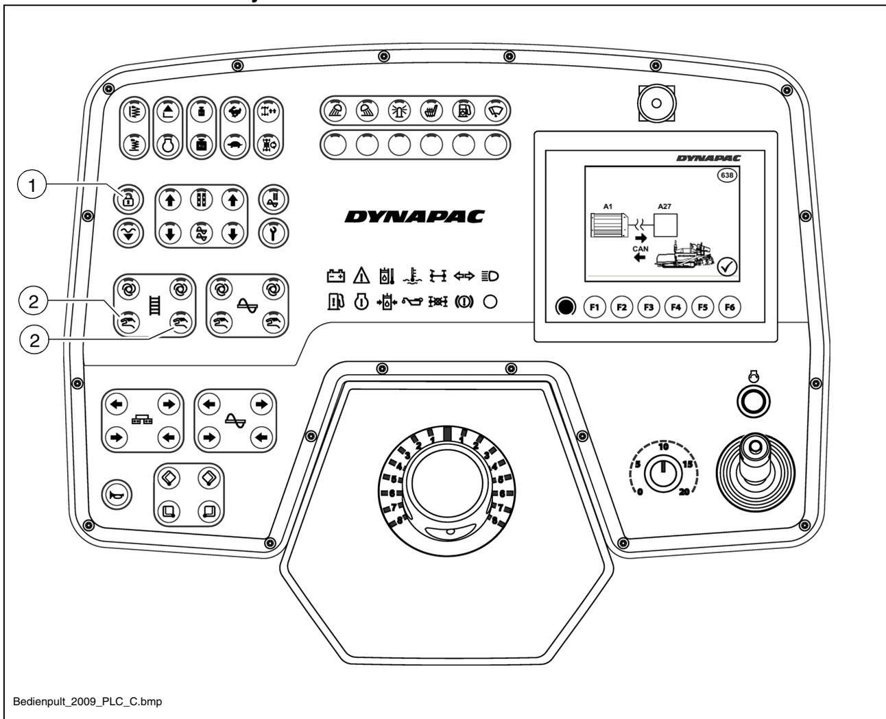
The conveyor's direction can be reversed in order to slightly reverse any paving material which may be positioned just in front of the auger. This enables e.g. material losses to be avoided during transportation.
