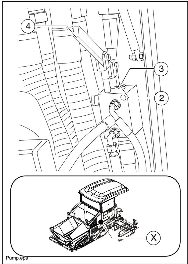
Following towing, unscrew the threaded dowel (3) a few turns again and lock with the lock nut (2).
