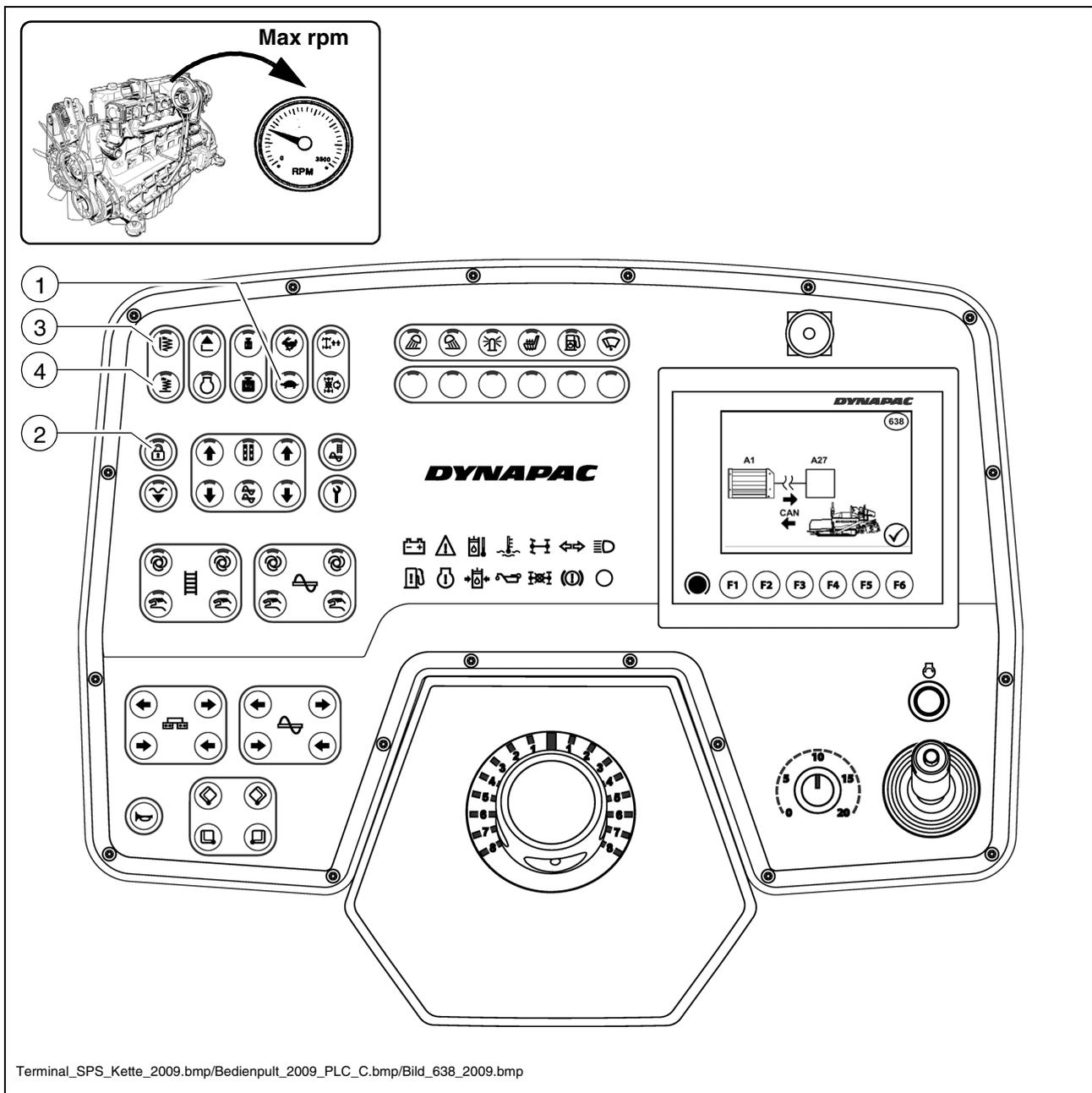
To guarantee temporary paver finisher operability in the event that the keyboard fails, an emergency programme is automatically started.
