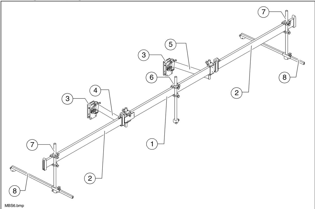
The big ski is used for contactless sensing over a particularly large reference length.
