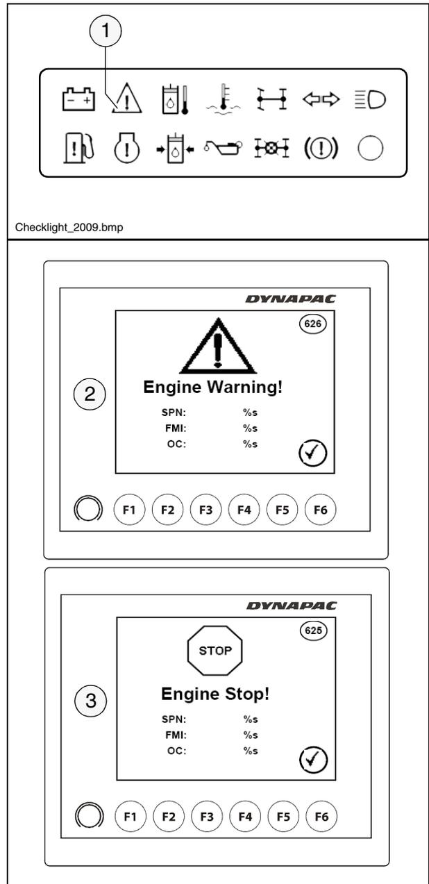
The error message simultaneously shown on the display contains several numerical codes, which uniquely define the fault after decoding.
