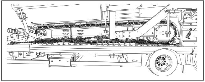
Diagonal lashing secures the paver finisher at the side using the lashing points on the paver finisher and on the low-load trailer.
