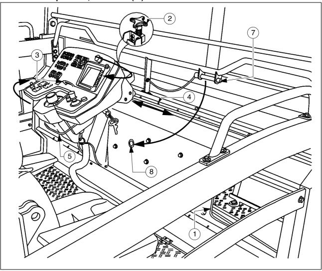
The control platform can be hydraulically shifted beyond the left/right outer edge of the vehicle, providing the driver with a better view of the paving area in this position.
