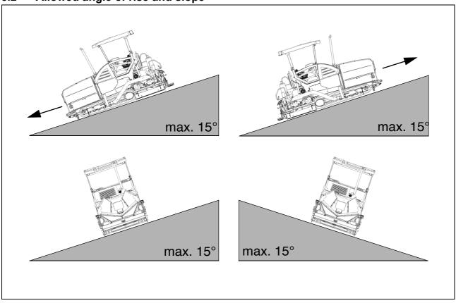
Before operating your vehicle in an inclined position (gradient, slope, lateral inclina-B tion) which is above the specified limit value, please consult the customer service department for your vehicle!
