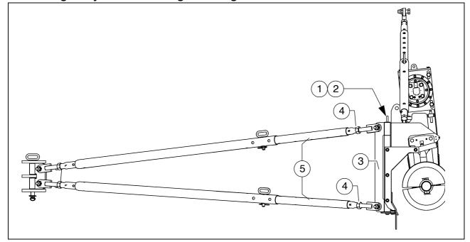
Auger height adjustment for large working widths can be carried out with a hinged brace:
