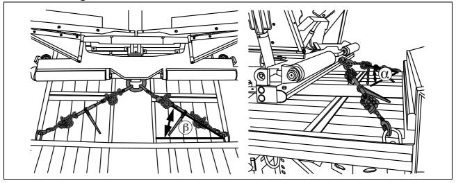
Diagonal lashing secures the paver finisher at the front using the lashing points on the paver finisher and on the low-load trailer. Fasten the lashing chains as shown.
