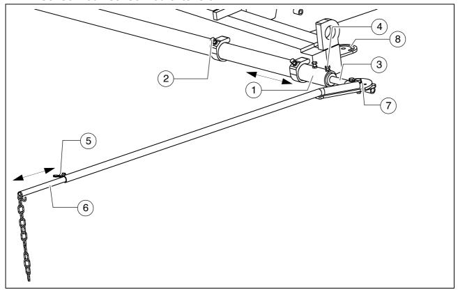
The sensor rod acts as an orientation aid for the vehicle driver during paving. Along the defined paving route, the vehicle driver can use the sensor rod to follow a tensioned reference wire or another marking.
