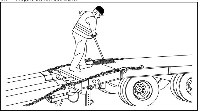
The floor of the loading space must always be undamaged, free of oil and mud, dry (residual moisture is permitted without accumulations of water) and swept clean!
