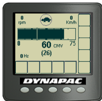
Fig. Compaction meter display (CMV display)
