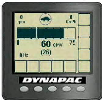
Fig. Compaction meter display (CMV display)
