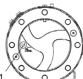
**Fig. Planetary gear/filling position**
