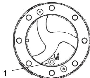
**Fig. Planetary gear/drainage position**
