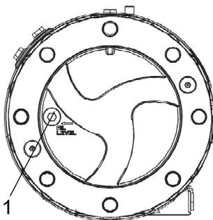
**Fig. Level check - planetary gear**
