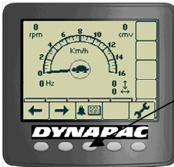
Alarms received are logged and can be seen by selecting Display alarms.
