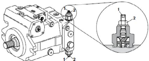
**Fig. Propulsion pump - By-pass valves**
