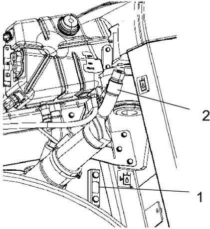
Place the roller on a level surface and check that the oil level in the sight glass (1) is between the max and min markings.
