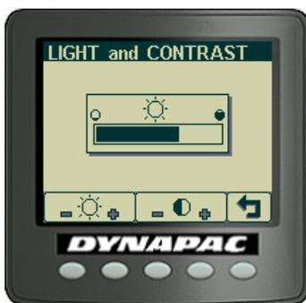
Adjustment of the light and contrast settings on the display, including brightness of the panel light.
