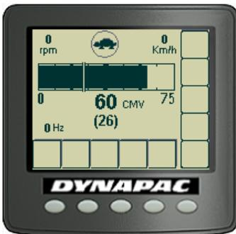
Fig. Compaction meter display (CMV display)
