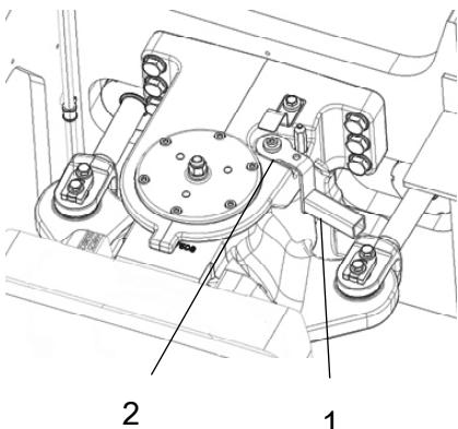
**Fig. Steering joint lock, locked**
