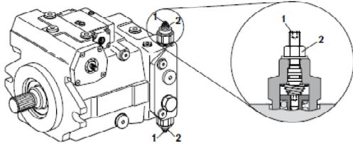
**Fig. Propulsion pump - By-pass valves**
