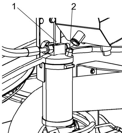
Fig. Drying filter in engine compartment
