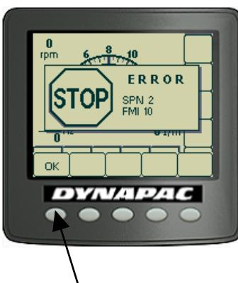
When an engine alarm is activated, the alarm is shown on the display.
