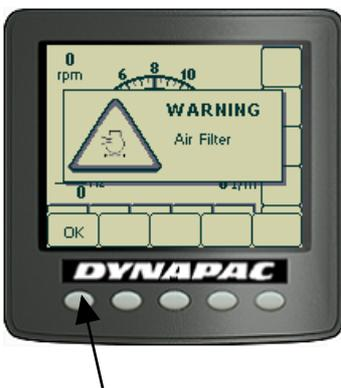
When a machine alarm is activated the alarm is shown on the display, plus a warning text that describes the alarm.
