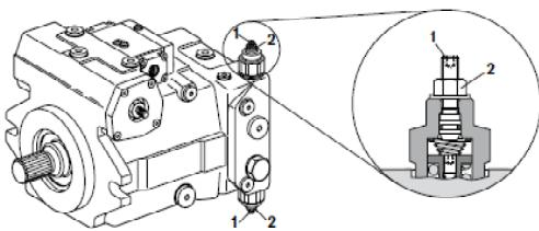
**Fig. Propulsion pump - By-pass valves**
