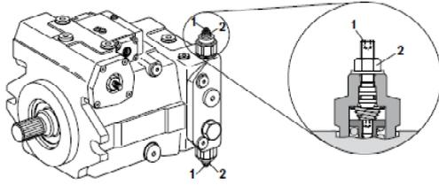
**Fig. Propulsion pump - By-pass valves**
