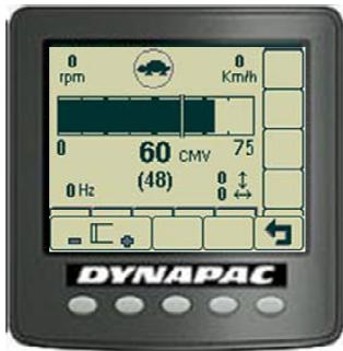
The compaction meter value view in display will give the operator all information needed during compaction; engine rpm, gear position, speed, frequency and inclinations are in display together with actual CMV and the limit set in brackets. Use the buttons underneath the display to set the limit. The scale will switch automatically depending on the CMV reading.
