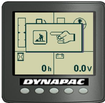
To activate the above functions it is necessary to make sure that the machine's Workmode is activated.
