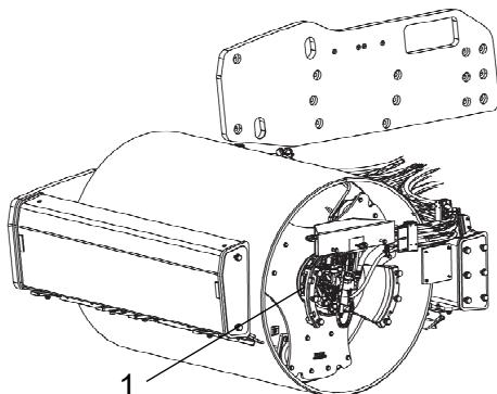
**Fig. Oil filling - drum gear**
