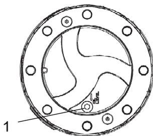
**Fig. Planetary gear/drainage position**
