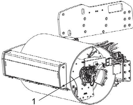
**Fig. Oil filling - drum gear**
