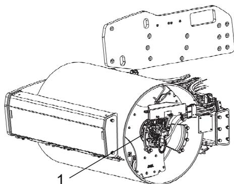
**Fig. Checking the oil level - Drum gearbox**
