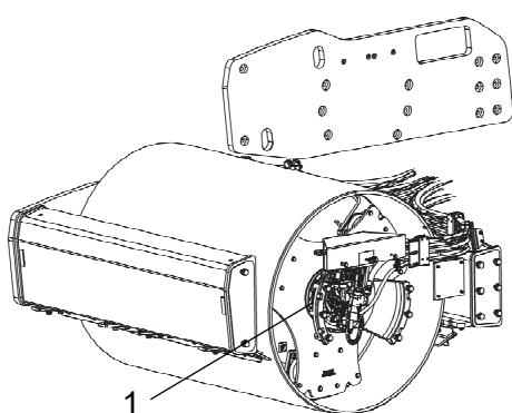
**Fig. Checking the oil level - Drum gearbox**
