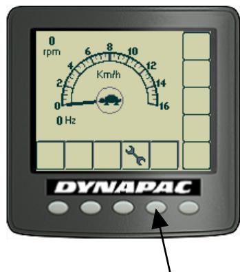
A Service symbol is now visible at the bottom of the display screen.
