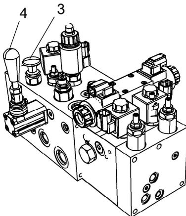
**Fig. Valve block, engine compartment**
