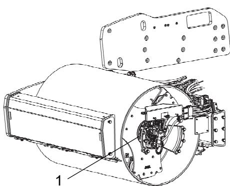
**Fig. Oil filling - drum gear**
