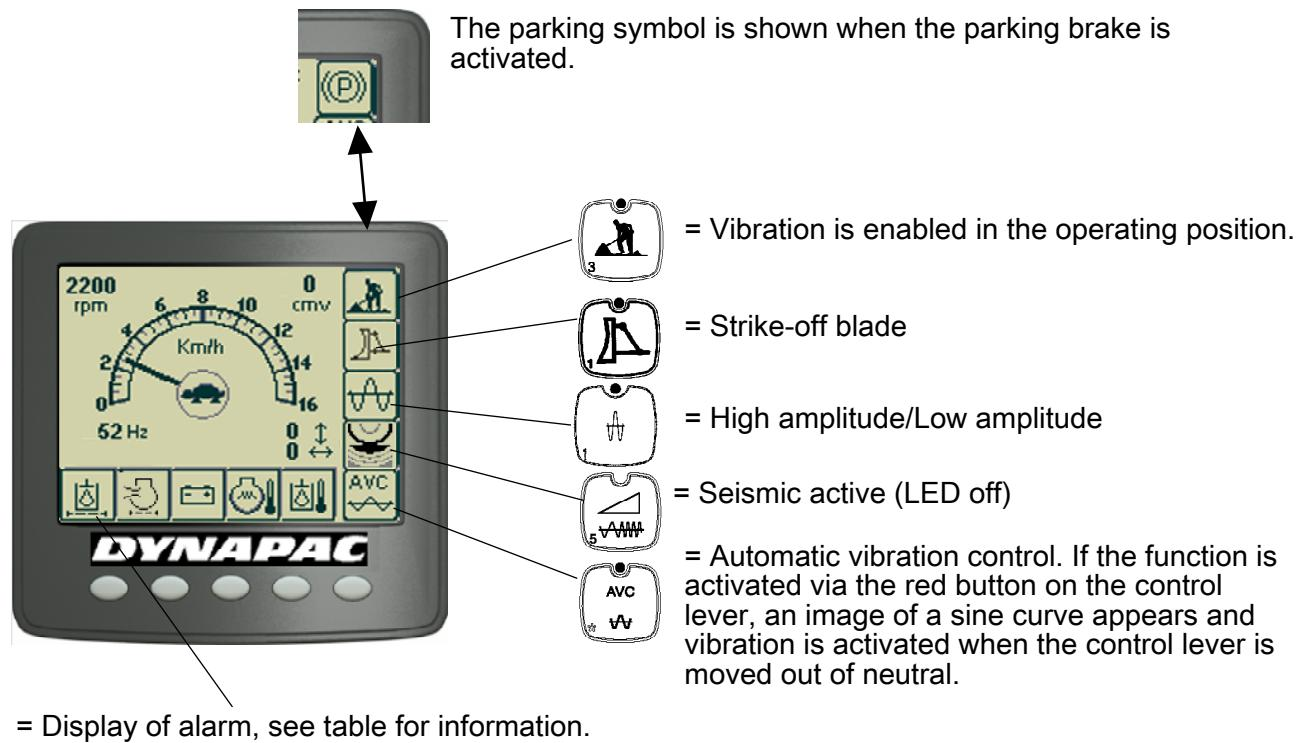
**Instruments and controls, cab**
