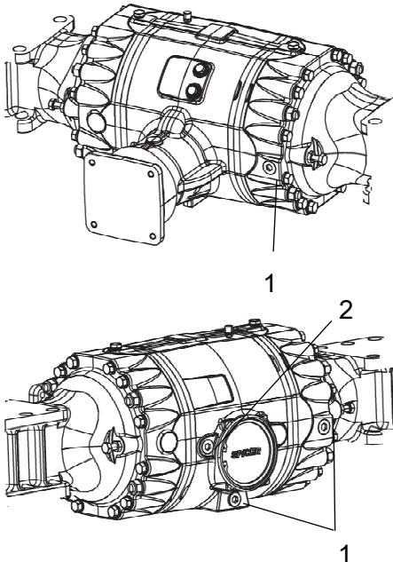
**Fig. Level control - differential housing**
