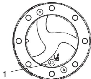
**Fig. Planetary gear/drainage position**
