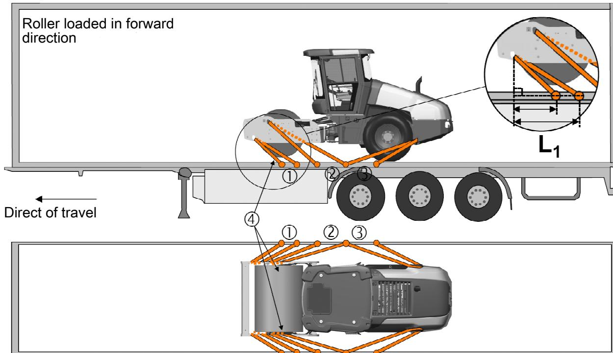
1 - 3 = double lashings, i.e. one lashing with two parts secured to two different lashing mounts, symmetrically located on the right and left sides.
