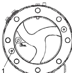
**Fig. Level check - planetary gear**
