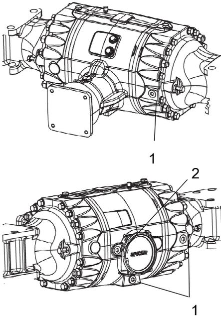
Wipe clean and remove the level plugs (1) and check that the oil level reaches the lower edge of the plug holes. The plugs can be found at the front or rear of the rear axle.
