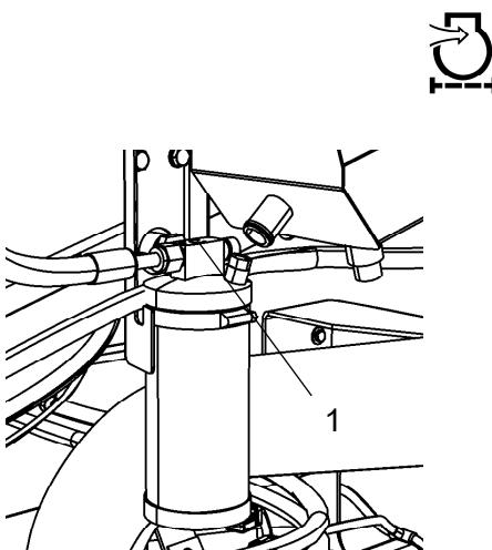
**Fig. Drying filter**
