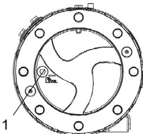
**Fig. Planetary gear/filling position**
