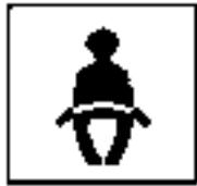
Unless the seat belt is used, a warning image appear in the display and a warning buzzer sounds to alert the driver to use the seat belt.
