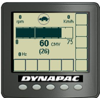
*Fig. Compaction meter display (CMV display)*
