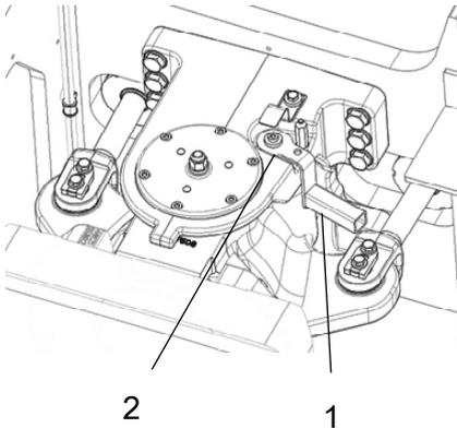
**Fig. Steering joint lock, locked**
