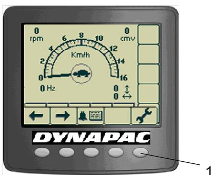
Fig. Main screen/Working screen with menu selection buttons (1)
