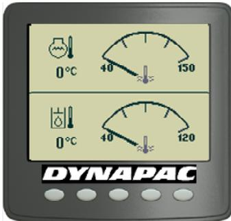
Fig. Temperature screen
