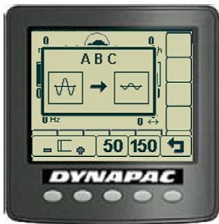
The analyzed information is presented in the display as a digital value expressed as CMV, Evib1 or Evib2. High or low measuring range is automatically selected and viewed in the display. The resulting numerical value is a relative measure of the ground stiffness achieved.
