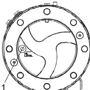
**Fig. Level check - planetary gear**
