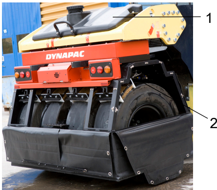
Fig. Wheel rack 1. Rear water tank 2. Sprinkler nozzle
