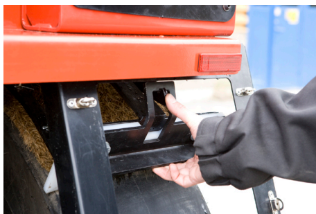
Fig. Wheel scrapers 1. Scraper blades 2. Locking hook
