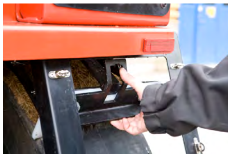
Fig. Wheel scrapers 1. Scraper blades 2. Locking hook
