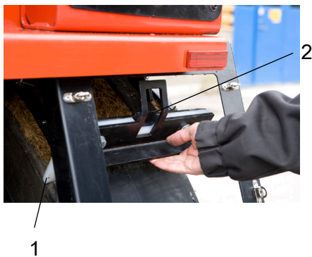
Fig. Wheel scrapers 1. Scraper blades 2. Locking hook
