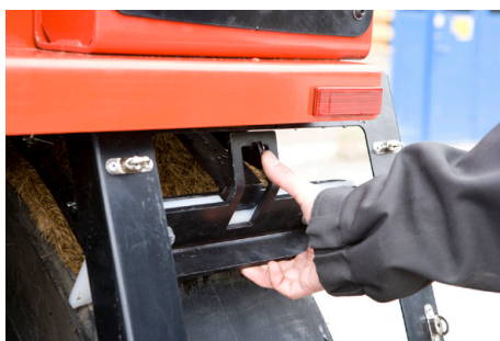
Fig. Wheel scrapers 1. Scraper blades 2. Locking hook
