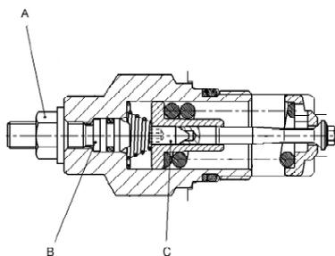
**Figure. Soupape de remorquage**
