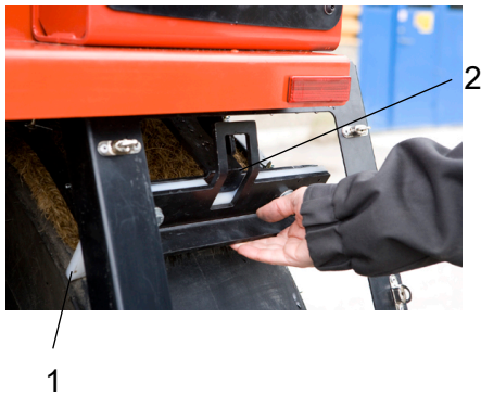
Fig. Wheel scrapers 1. Scraper blades 2. Locking hook
