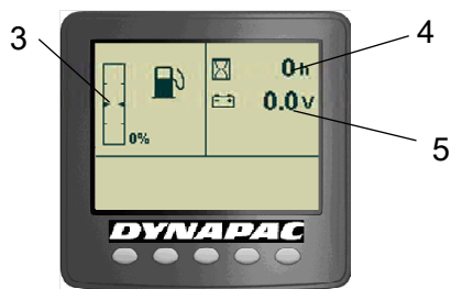
Fig. Status image 3. Fuel level 4. Hourmeter 5. Voltmeter
