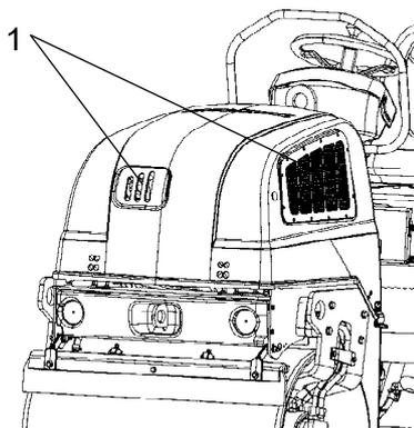
**Fig. Capota do motor**
