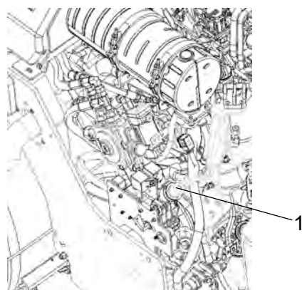
Fig. Engine compartment 1. Hydraulic fluid refilling
