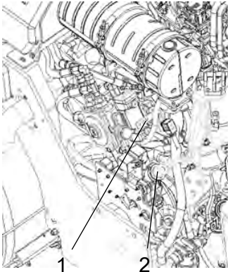
Fig. Engine compartment 1. Forward/Reverse lever 2. Hydraulic reservoir cap
