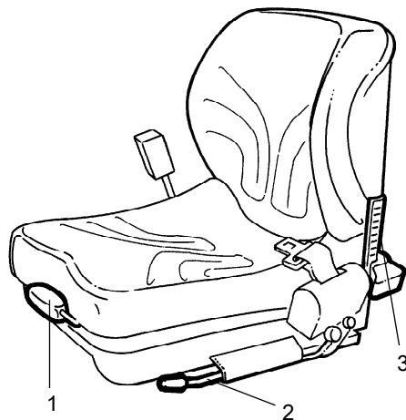
Fig. Operator position 1. Backrest inclination 2. Length adjustment 3. Weight adjustment
