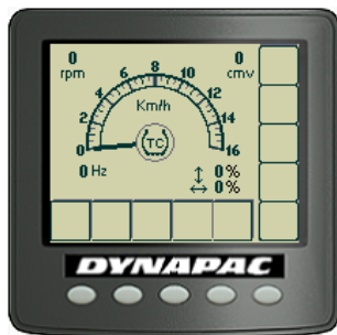
Fig. The display shows whether TC (Anti-spin) is activated or disengaged
