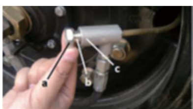
Fig 4. 1. Lock nut; 2. Valve element 3. Valve body
