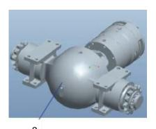
Fig. Level check – driving gear 3. Level plug
