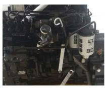
Fig. Filter unit Pre filter + Fuel filter
