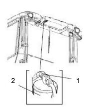
Fig. Drying filter 1. Sight glass
