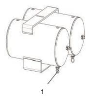
Fig. Drain valve
