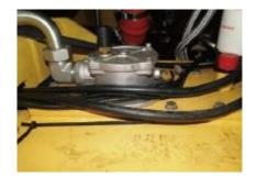
Fig. Hydraulic fluid filter
