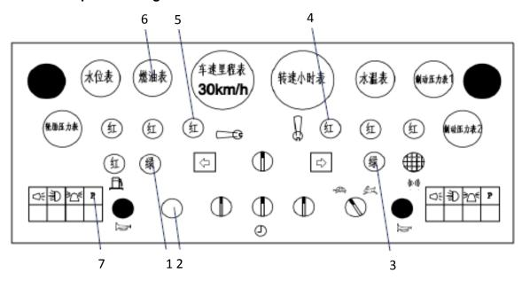
Turn the ignition key (2) to "ON" position, neutral position indicator (5), parking indicator (4) and control indicator (1) or (3) on operator side are all activated.
