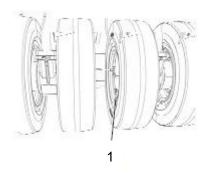
Fig. Inner wheels 1. Air valve
