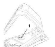
Fig. Water tank 1.Drain cock
