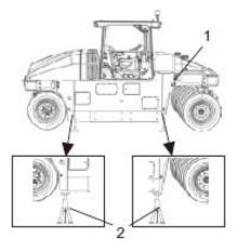
Fig. Roller lifted with jack
