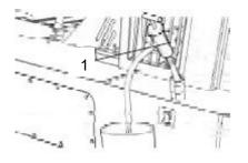
Fig. Fuel tank 1.Oil drain pump
