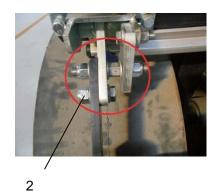
The distance can be adjusted easily by through the fixing bolts (2) of the bracket to avoid over spraying beyond tire or missing spray.
