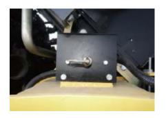
Fig. Engine compartment1. Battery disconnector
