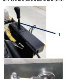
To start the machine the forward/backward lever must be in neutral position, in the middle.
