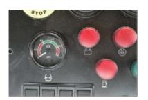
Check the air pressure from the air gauge on instrument panel, it should be in 380kPa - 780kPa. (fig1).
