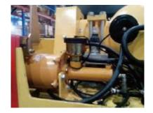
Fig. Brake fluid container
