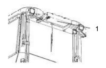
Fig. Cab 1. Condenser element
