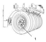
Fig. Outer wheels 1. Air valve
