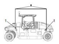
Fig. Roller prepared for lifting
