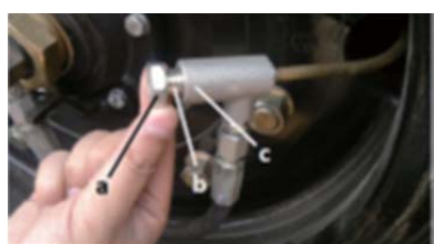
Fig 4. 1. Lock nut; 2. Valve element 3. Valve body
