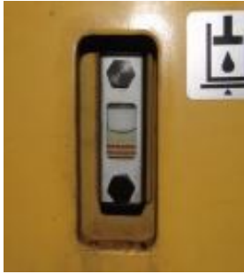
Fig. Hydraulic reservoir
