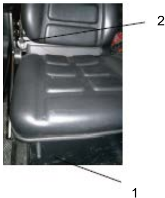
Fig2. Driver seat 1. Locking lever – Length adjustment 2. Backrest angle
