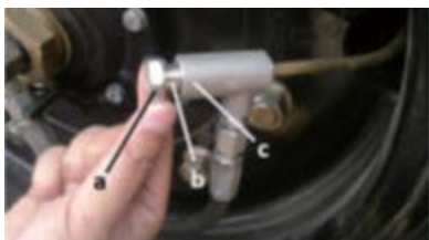
Fig 4. 1. Lock nut; 2. Valve element 3. Valve body
