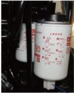
Fig. Fuel filter 1. Drain plug
