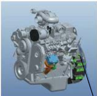
Fig. Engine compartment 1. Dipstick
