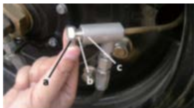
Fig 4. 1. Lock nut; 2. Valve element 3. Valve body
