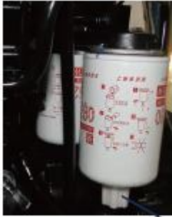
Fig. Fuel filter 1. Drain plug
