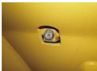
Fig. Hydraulic reservoir drain plug
