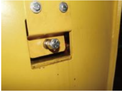
Fig. Drain plugs
