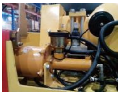
Fig. Brake fluid container
