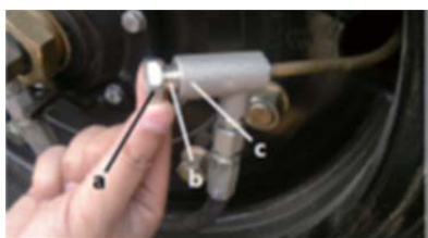
Fig 4. 1. Lock nut; 2. Valve element 3. Valve body
