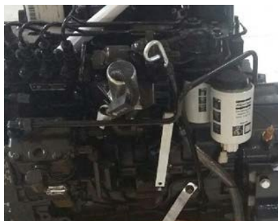
Fig. Filter unit Pre filter + Fuel filter
