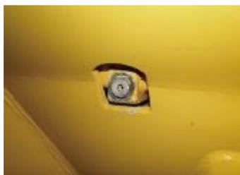
***Fig. Hydraulic reservoir drain plug***
