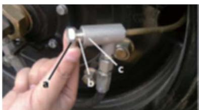
Fig 4. 1. Lock nut; 2. Valve element
