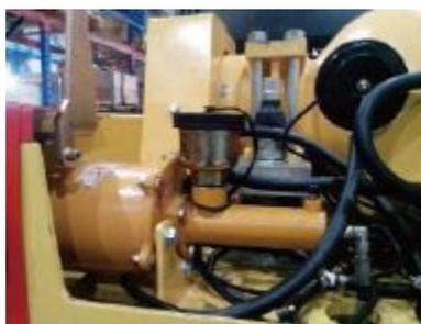
**Fig. Brake fluid container**
