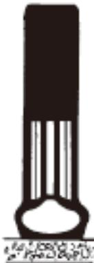
**Fig. Low ground pressure, larger area**
