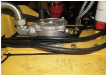
**Fig. Hydraulic fluid filter**
