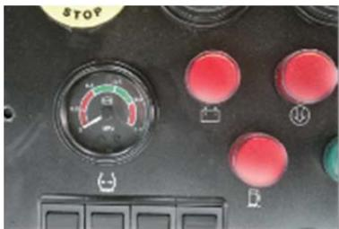
Fig 1. Instrument panel – Air gauge
