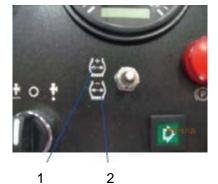
Fig1. Control panel1. Tire pressure (+)2. Tire pressure (-)
