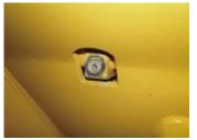
Fig. Hydraulic reservoir drain plug
