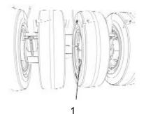
Fig. Inner wheels 1. Air valve
