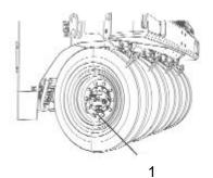
Fig. Outer wheels 1. Air valve
