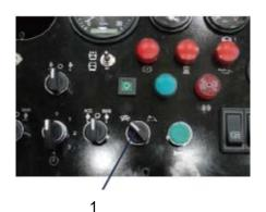
While roller is stationary, change the direction or change gears.
