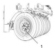
Fig. Outer wheels 1. Air valve
