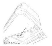
Fig. Water tank 1.Drain cock
