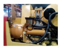
Fig. Brake fluid container
