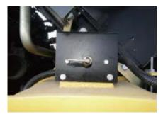
Fig. Engine compartment1. Battery disconnector
