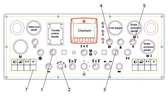
Turn the ignition key (2) to "ON" position, neutral position indicator (5), parking indicator (4) and control indicator (1) or (3) on operator side are all activated. Make sure the parking brake button (7) is on "pressed" condition.
