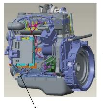
Fig. Engine compartment 1. Dipstick The dipstick is located under the engine hood. Take care not to touch any hot parts of the engine or radiator when removing the dipstick. Risk of burns.
