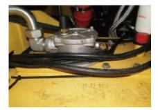
Fig. Hydraulic fluid filter
