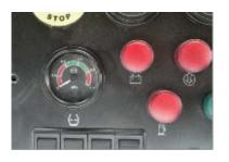
Check the air pressure from the air gauge on instrument panel, it should be in 380kPa – 780kPa. (fig1).
