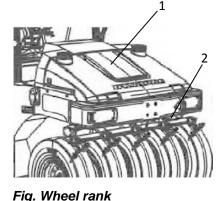
Fill the tank with emulsion fluid, e.g. water mixed with 2% cutting fluid. Check that the sprinkler nozzles (2) are not blocked, and if necessary clean them and the filter. See under Sprinkler system, Check – Cleaning, for detailed instructions.
