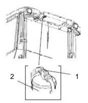
Fig. Drying filter 1. Sight glass 2. Filter holder Air conditioning (Optional) – Drying
