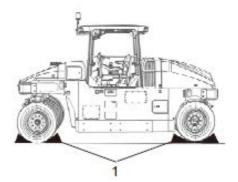
Fig. Chocking the wheels 1. Chocks
