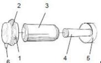
Change the air cleaner main filter when the warning lamp on the control panel comes on when the engine is running at maximum speed.
