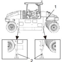
Fig. Roller lifted with jack
