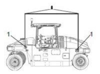
Fig. Roller prepared for lifting 1. Hoisting plate
