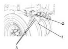
Fig. Tire scrapers 1-2mm
