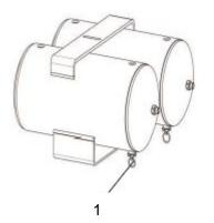
Fig. Drain valve
