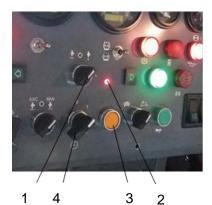
Switch on the battery switch;
