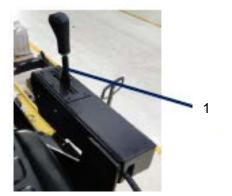
To start the machine the forward/backward lever must be in neutral position, in the middle.
