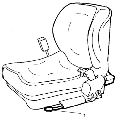
Fig. Operator's seat 1. Length adjustment
