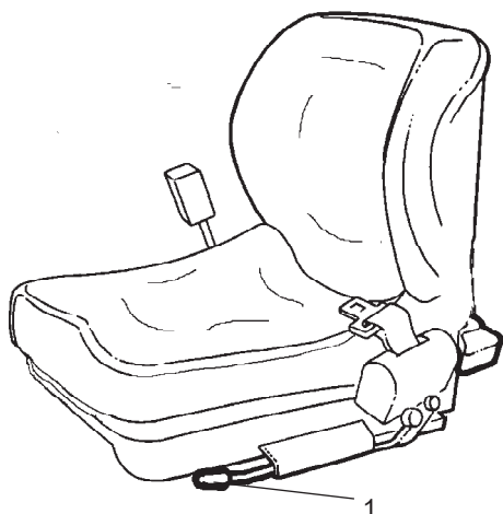
Fig. Operator's seat 1. Length adjustment
