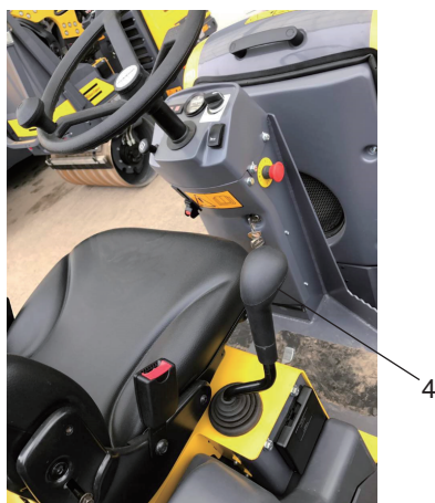
Fig. Forward/Reverse lever 4. Switch, vibration On/Off
