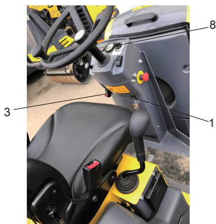
Figure. Instrument panel 1. Ignition key 3. Parking brake 8. Switch, sprinkler
