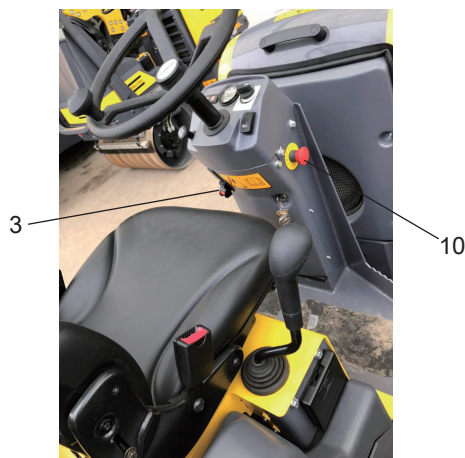
Fig. Controls 3. Parking brake 10. Emergency stop
