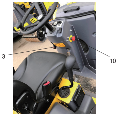
Figure. Control panel 3. Parking brake 10. Emergency stop
