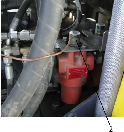
Fig. High pressure hydraulic filter 1. Filter indicator
