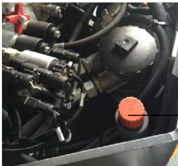
Fig. Hydraulic reservoir
