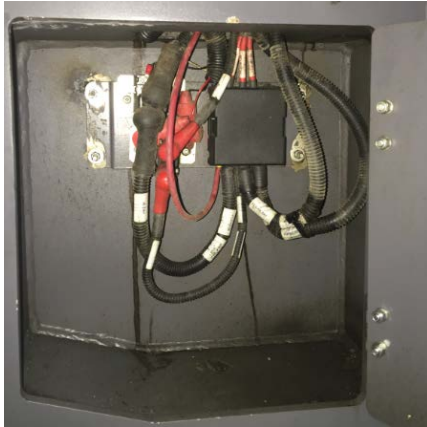
Fig. Engine compartment, positioning of main fuses.
