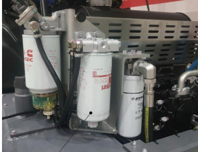
4 Fig. 1. Fuel filter 4. Pre-Fuel filter (NOTE: CA50 W/O)
