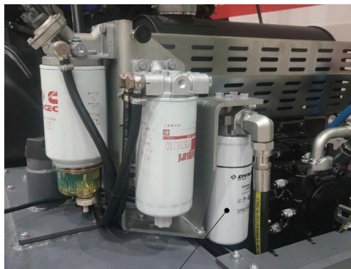
Fig. Engine compartment: 1. Hydraulic fluid filter.
