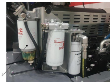
4 Fig. 1. Fuel filter 4. Pre-Fuel filter (NOTE: CA50 W/O)
