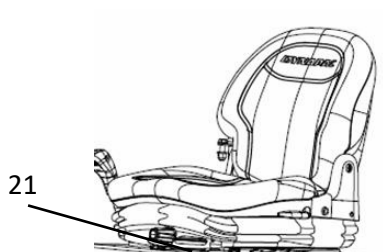
Fig. Operator's seat 21. Length adjustment
