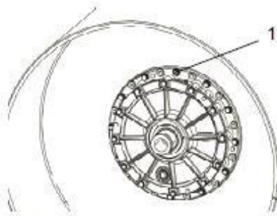
Fig. Drum 1. Ventilation screw
