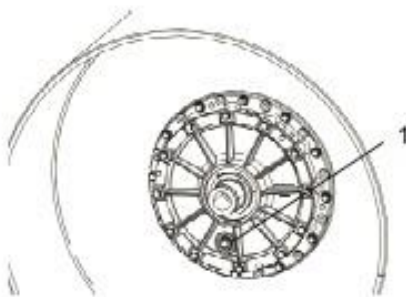
Fig. Drum 1. Oil level glass
