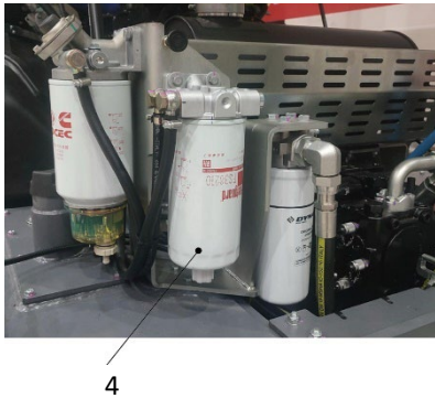
Fig. 1. Fuel filter 4. Pre-Fuel filter (NOTE: CA50 W/O)
