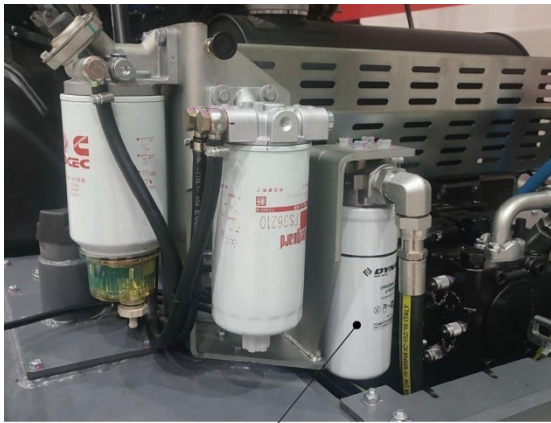
Fig. Engine hood rear left side 1. Hydraulic fluid filter.
