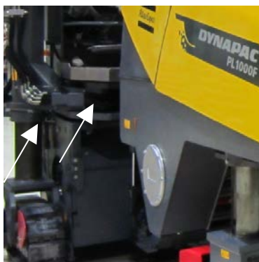
Fig. Rear right chassis leg, lubrication point
