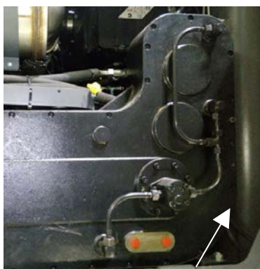
Fig. Rear left chassis leg, lubrication point
