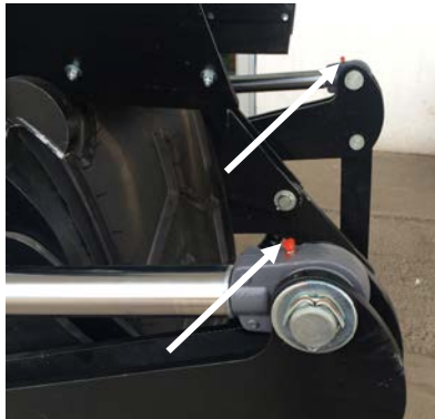
Fig. Discharge conveyor, folding cylinder
