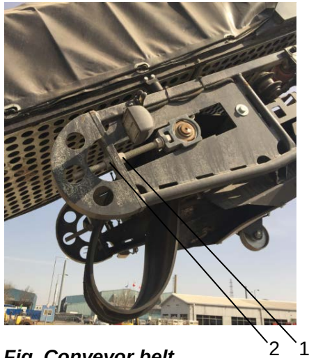
Fig. Conveyor belt Belt tension 1.Lock nuts 2.Adjuster nuts
