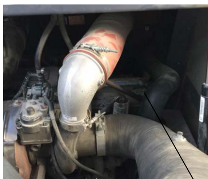
Fig. 1. Engine oil filter 2. Drain cock 3. Engine oil filler
