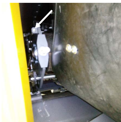
Fig. Primary conveyor, drive, grease nipple
