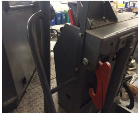
Fig. Locking device, scraper 1. Lock handle
