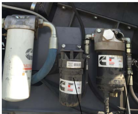
Fig. Fuel filter 1. Ball valve 2. Fuel filter
