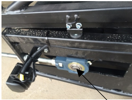
Fig. Conveyor, tension bearing, grease nipple
