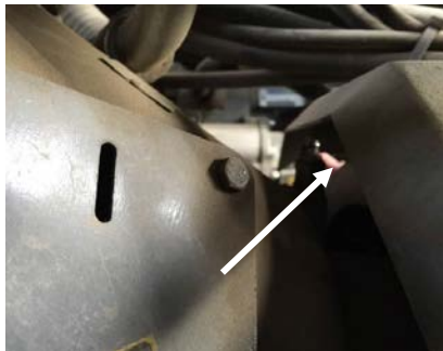
Fig. Clutch bearing, grease nipple
