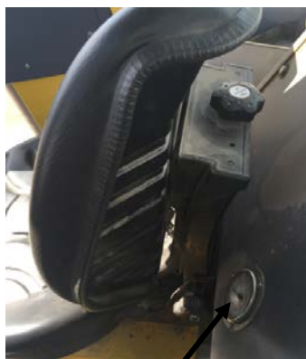
Fig. Manometer, scraper release pressure
