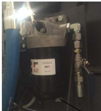
Fig. Fuel prefilter 1. Drain valve
