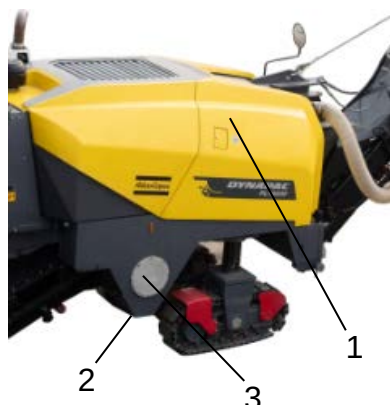
Fig. 1. Fuel tank 2. Drain plug 3. Cover
