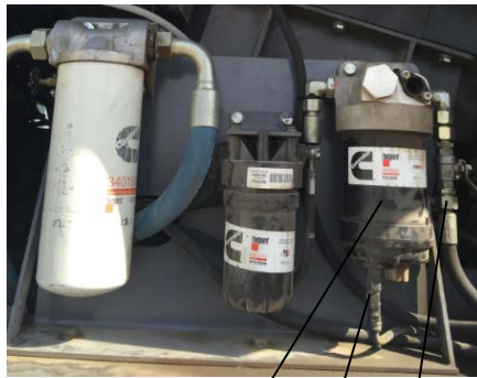
Fig. 1. Ball valve 2. Sensor 3. Filter cartridge
