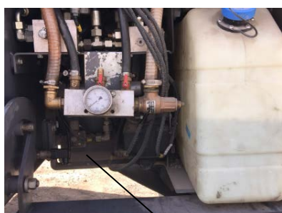
Fig. Water filter 1. Filter element, strainer
