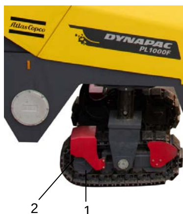
Fig. Planetary gear/position for filling
