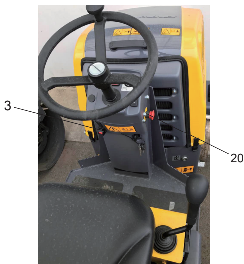
Figure. Control panel 3. Parking brake 20. Emergency stop
