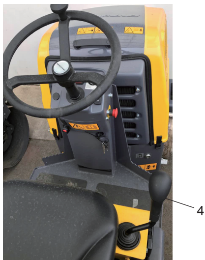
Fig. Forward/Reverse lever 4. Switch, vibration On/Off
