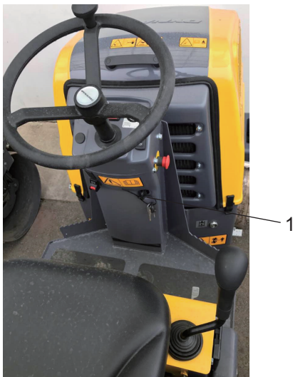
Fig. Instrument panel 1. Starter switch
