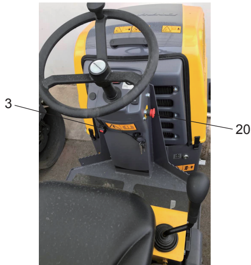
Fig. Controls 3. Parking brake 20. Emergency stop
