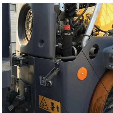
Figure. Under the engine compartment 1. Hydraulic fluid tank cap 2. Hydraulic oil level
