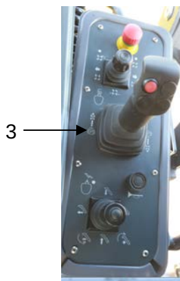
Fig. Switch panel, ergo control panel
