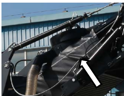
Fig. Steel retaining cables
