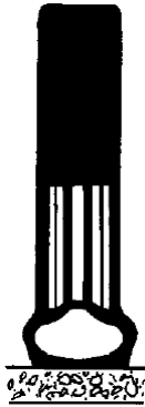
Fig. - Low ground pressure, larger contact area
