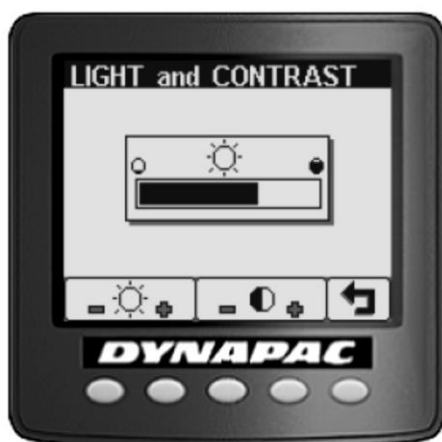
Fig. – Brightness and contrast screen
