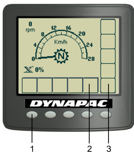
Fig. – Operation main screen with the menu selection buttons
