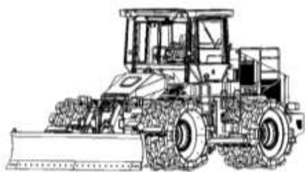
Fig. - Tamping roller with leveling blade
