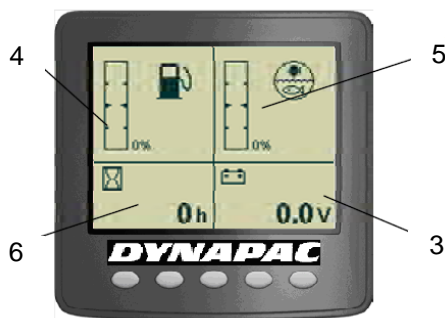
Fig.- Status screen 3. Voltmeter 4. Fuel level 5. Water level 6. Hourmeter
