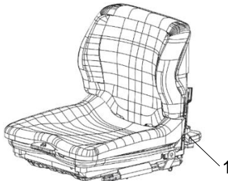
Fig. Operator's seat 1. Longitudinal adjustment
