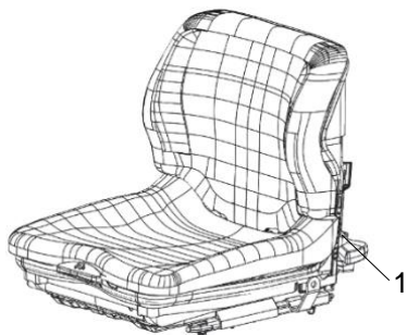
Fig. Operator's seat 1. Longitudinal adjustment
