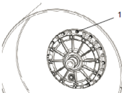
Fig. Drum 1. Ventilation screw
