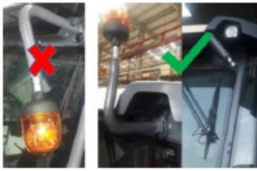
Fig. Orientation of Rotating Beacon
