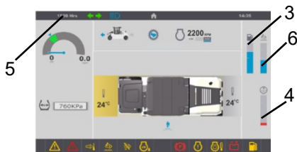
Fig. - Status image 3. Fuel level 4. Water level 5. Working hours 6. DEF level
