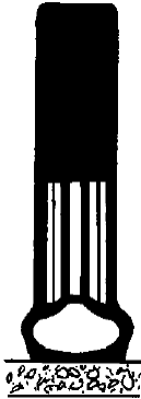
Fig. - Low ground pressure, larger contact area
