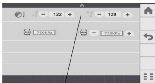
Asphalt Temperature Sensor Adjustment (Minimum and Maximum)
