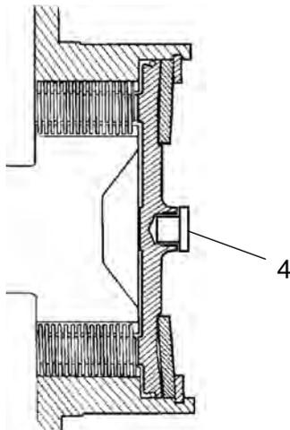
**Fig. Brake housing**
