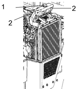
**Figure. Cooling water container**
