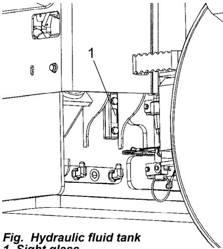
**Fig. Hydraulic fluid tank**
