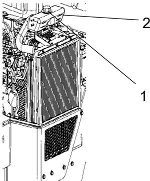
**Figure. Cooling water container**
