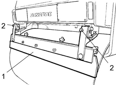
**Fig. Spring-action scrapers**
