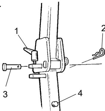
**Fig. ROPS locking device**
