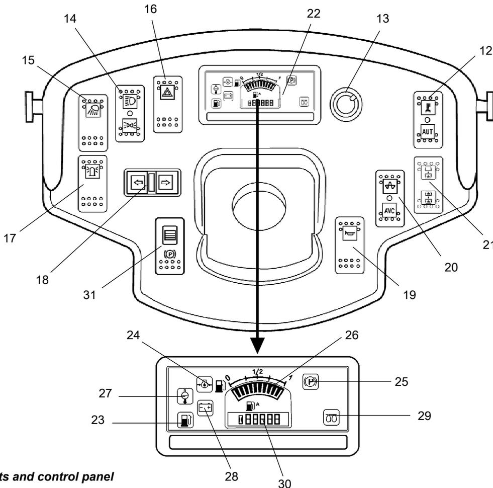
Fig. Instruments and control panel
