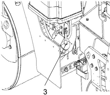
**Fig. Hydraulic oil filter**
