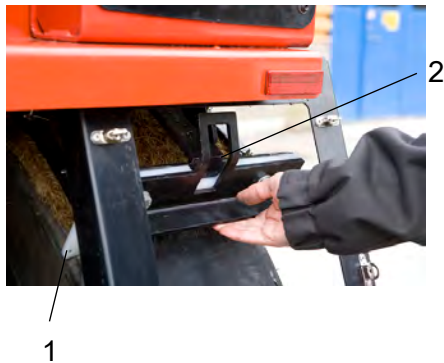
Fig. Wheel scrapers 1. Scraper blades 2. Locking hook
