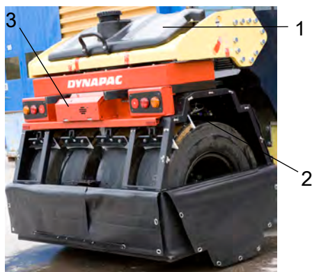
Fig. Wheel rack 1. Rear water tank 2. Sprinkler nozzle 3. Sprinkler system
