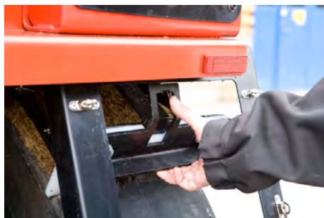
Fig. Wheel scrapers 1. Scraper blades 2. Locking hook
