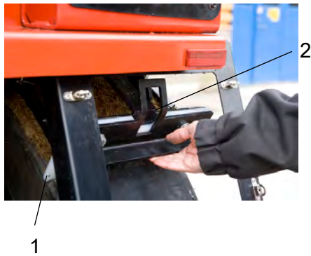
Fig. Wheel scrapers 1. Scraper blades 2. Locking hook
