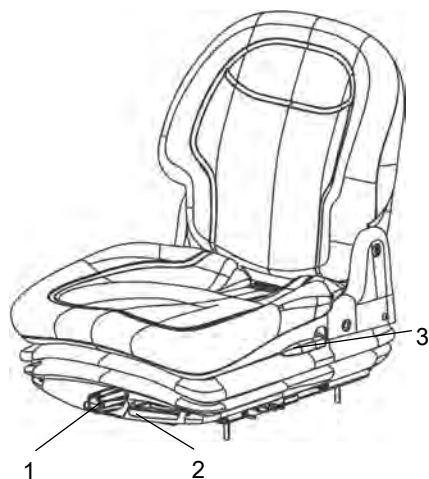
Fig. Operator position 1. Backrest inclination 2. Length adjustment 3. Weight adjustment
