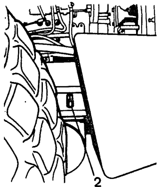
Fig 31 Draining the engine oil
