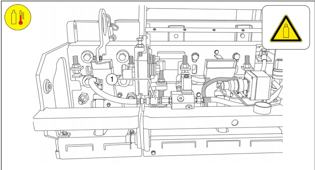
After the extension parts have been mounted, the connection hoses for the extension parts' burners must be connected to the screed's pipe system.
