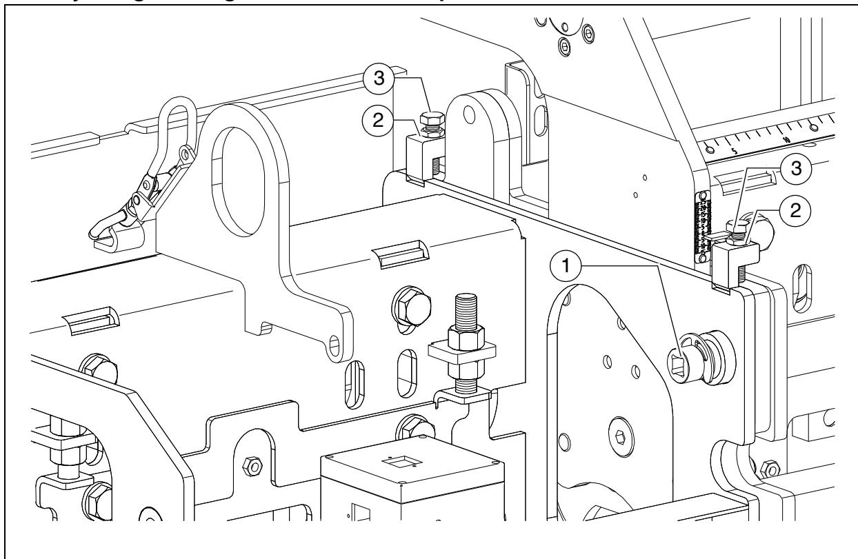
To ensure that the screed paves without marks and the extension parts can also be adjusted to the various operating conditions during use, the height of the extension parts can be adjusted:
