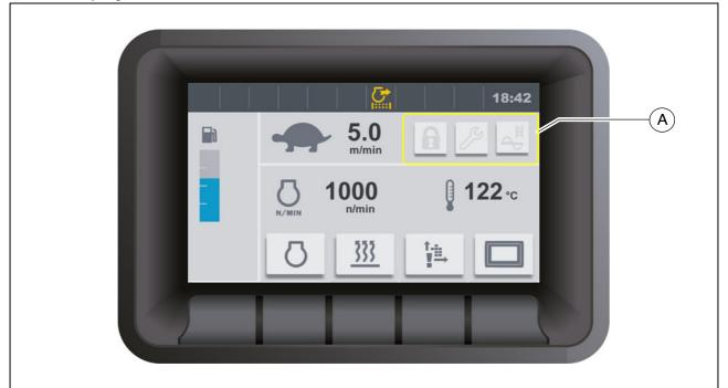
Some functions switched on with the operating panel are shown for confirmation in the display area (A). The function is activated when the corresponding symbol appears blue.
