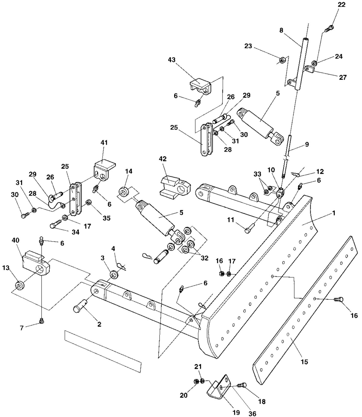
Levelling blade, metal parts
