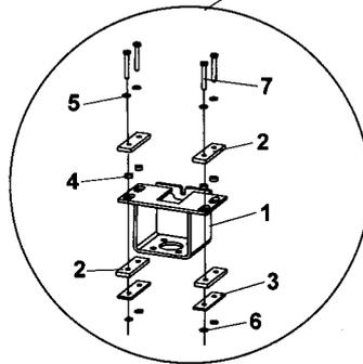
**Bracket, Steering valve vibration isolated Option**
