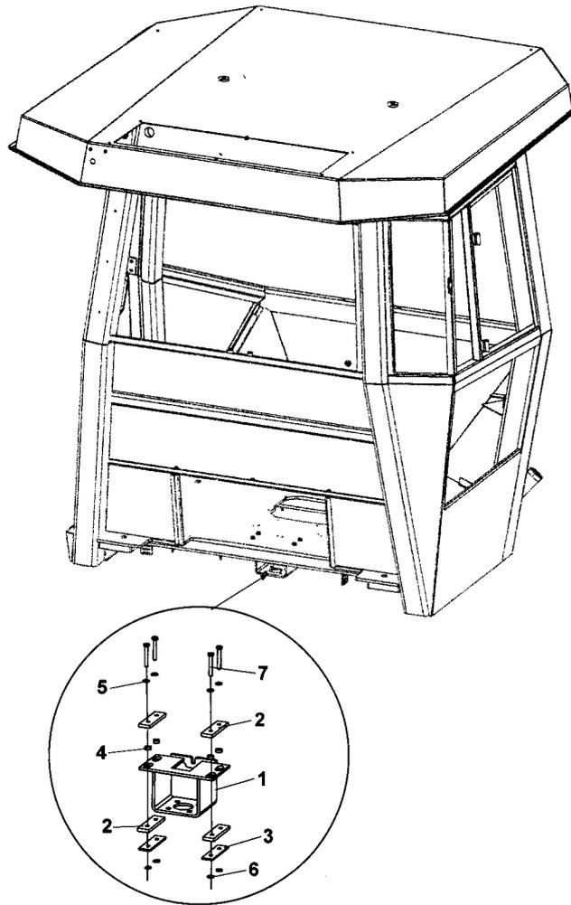
**Bracket, Steering valve vibration isolated Option**
