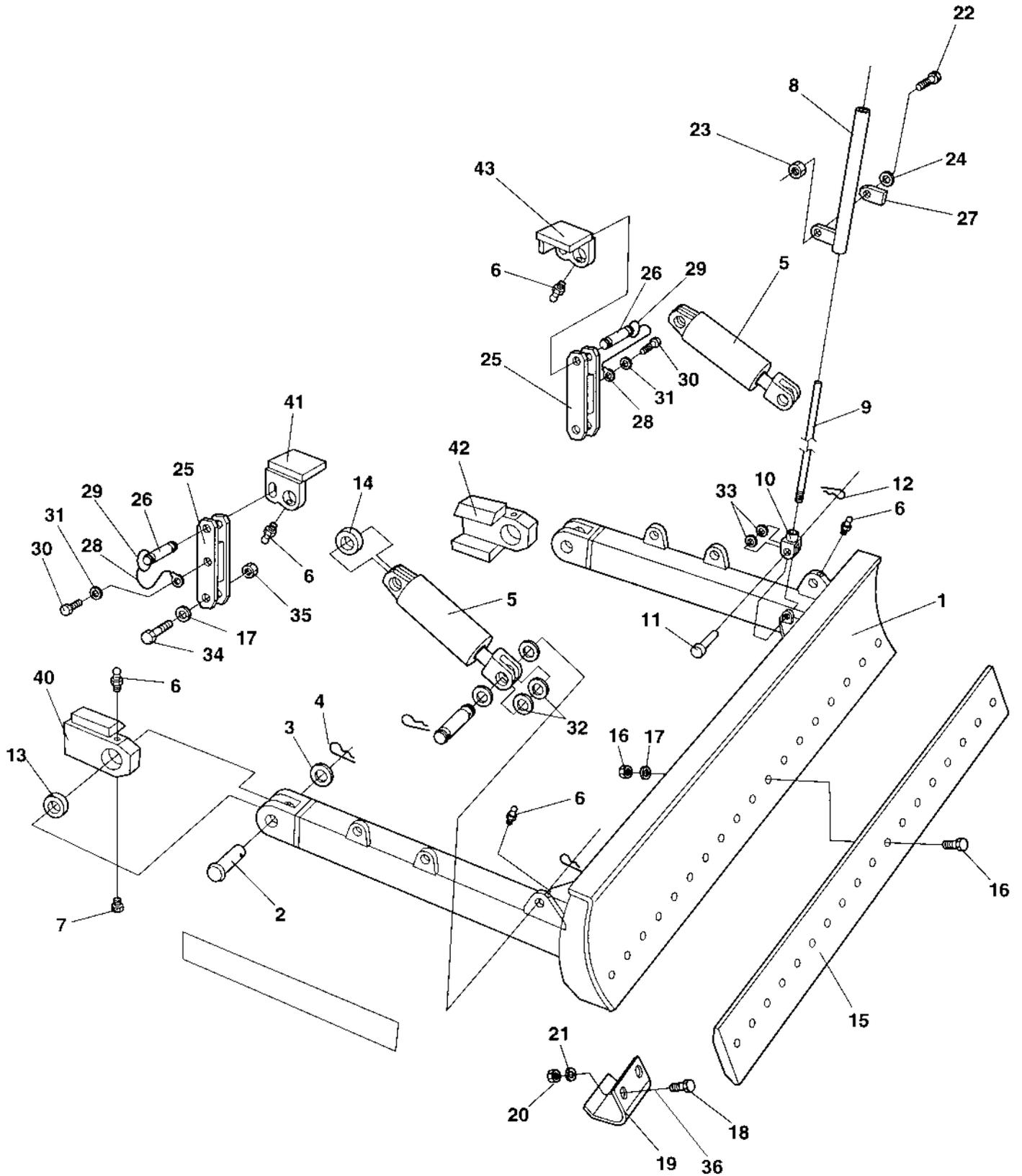
Levelling blade, metal parts
