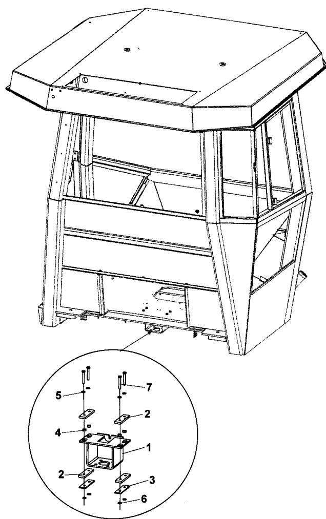
**Bracket, Steering valve vibration isolated Option**
