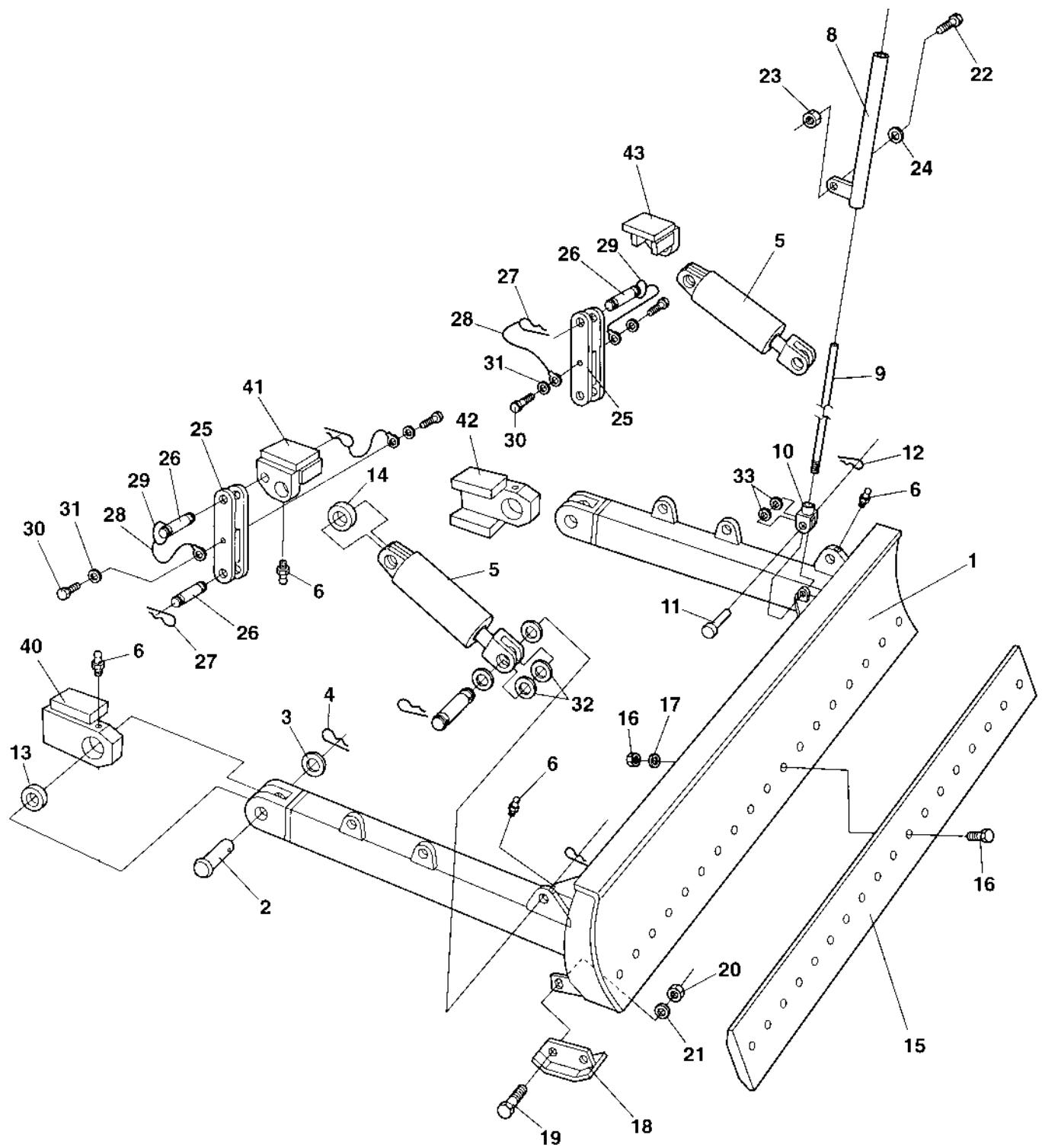
**Levelling blade, metal parts**
